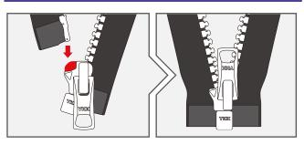
Enlarged bottom part of slider body (highlighted in red) allows quick and easy insertion of the separable pin into the slider.
